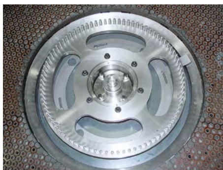
Measuring anvil, inner pin ring and segmented grinding wheel
