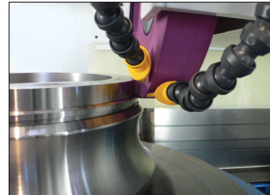
Picture 12: Face grinding
