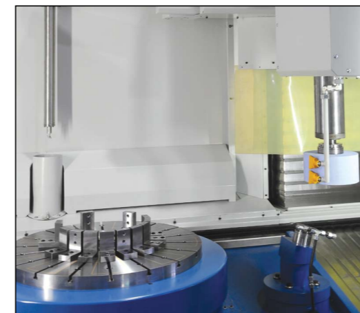
Picture 6: Revolver with four tool stations and measuring system
