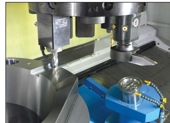
Picture 14: Milling of a horizontal flute
