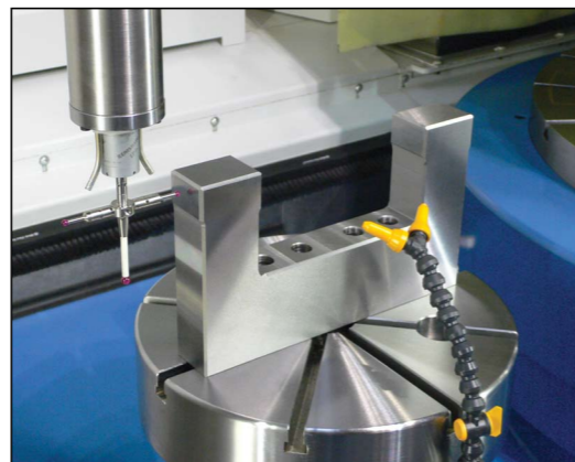
Picture 10: In-process calibration of the probe
