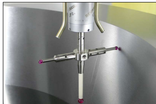
Picture 10: In-process measuring
