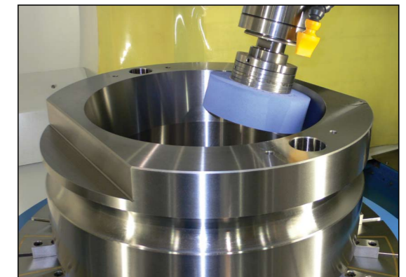
Picture 15: Internal taper grinding
