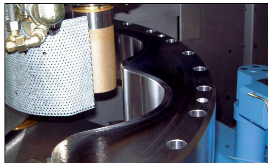
Picture : Grinding of an internal contour
