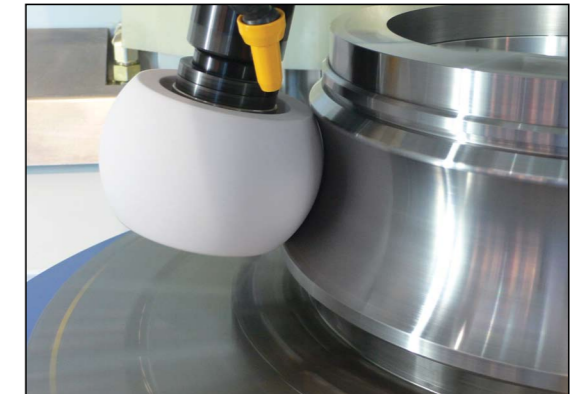
Picture 13: Grinding of an external contour
