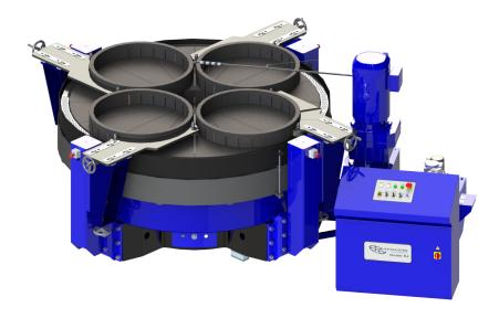
The Lapmaster Wolters Model 84 is equipped with a 2134mm diameter lap plate. This is manufactured from Grade 300 grey cast iron to ISO 185(2005). It consists of individual segments bolted to a support plate.
