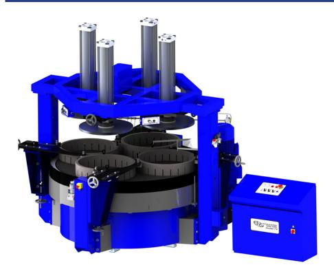
The Lapmaster Wolters model 72 is equipped with a 1829mm diameter lap plate. This is manufactured from Grade 300 grey cast iron to ISO 185(2005). It consists of individual segments bolted to a support plate.
