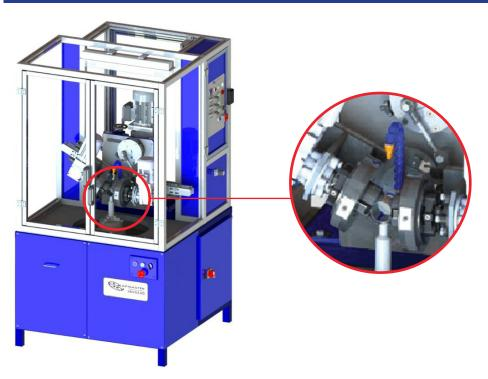
The Lapmaster LBVS ball valve lapping machine has been developed to maintain very accurate spherical surfaces on a variety of Ball Valves. The machine match laps two Seats to the valve, achieving a perfect mechanical seal for any pressure requirement.
