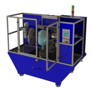
The Lapmaster Wolters LBVS ball valve lapping machine has been developed to maintain very accurate spherical surfaces on a variety of Ball Valves. The machine match laps two Seats to the valve, achieving a perfect mechanical seal for any pressure requirement.
