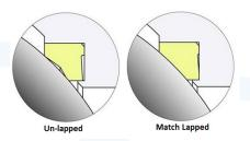
This system is effective on most materials including ceramic, graphite, ferrous metals, alloyed metals and sterlite coatings.
