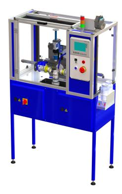
The Lapmaster LBVS ball valve lapping machine has been developed to maintain very accurate spherical surfaces on a variety of Ball Valves. The machine match laps two seats to the valve, achieving a mechanical seal for a wide variety of pressure requirements.
