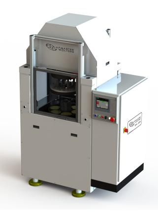
The Lapmaster DFL400 dual face lapping, polishing and fine grinding machine is based on a 3 way planetary concept, designed to yield precise and repeatable results at an economical price. Excellent results are obtained in the processing of a wide range of component materials including glass, ceramics, crystals and ferrous materials.
