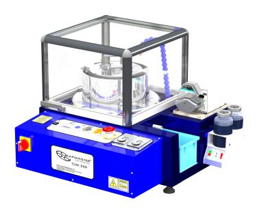
The Lapmaster Cylindrical Lapping machine is used to produce very accurate cylindrical surfaces on a large variety of components including Dowels, Rods and Roller bearings. Cylindrical lapping is a batch mode, loose abrasive machining process by which small amounts of material are removed from the OD of the work piece (about 0.01mm max), typically after an OD grinding operation. This process is designed to improve roundness and surface finish.
