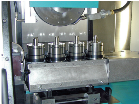
Grinding compartment with clamping fixture
