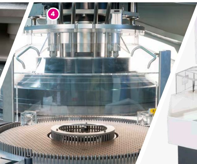
Upper Working Wheel With Safety Guard
