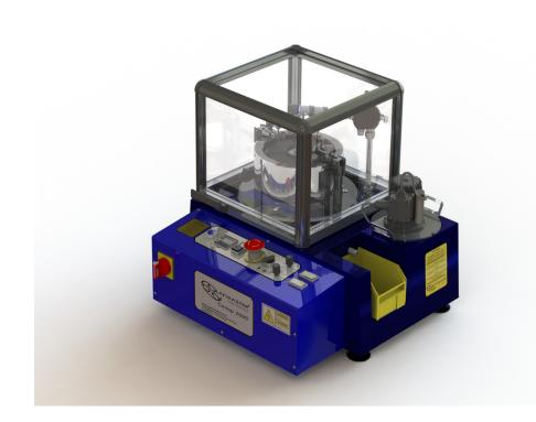
The Lapmaster-Wolters model 2000 machine is a small but versatile bench mounted machine ideally suited for small workshops and laboratories.
