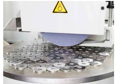
Grinding of a table load of small work pieces
